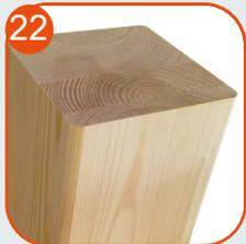
22 Posts made from coniferous wood, with a crosssection of 140x140 mm composed of 8 layers bonded with waterproof polyurethane adhesives. Undergoing a two step wood finishing system.
