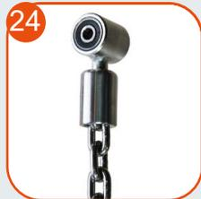
24 Swing slings, with double bearings, made of stainless steel guarantees a quiet mechanism operation. Beside the horizontal movement it allows as well for the circular movement to avoid twisting of the chain.
