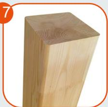
17 Posts made from coniferous wood, with a crosssection of 90x90 mm composed of 5 layers bonded with waterproof polyurethane adhesives. Undergoing a two step wood finishing system.
