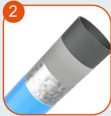
2 Solid construction made of black steel S235JR, cleaned in the sandblasting process. All elements made of black steel are subjected to a two-layer powder coating process, which includes the following stages: First layer - zinc-rich primer, Second layer - topcoat in RAL colour
