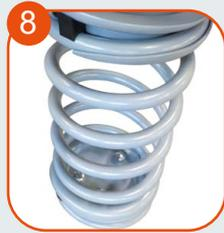
8 Springers' springs made of spring steel. The diameter of the spring is 200 mm and the diameter of the rod is 20 mm. The springs are subjected to a two-layer powder coating process, which includes the following stages: First layer - zinc-rich primer, Second layer - topcoat in RAL colour The fastenings are designed especially for solutions used on a playground, so they are stripped of elements which can cause danger to children
