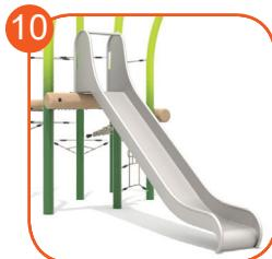
Slide made of stainless steel AISI 304. The metal sheet is 2 mm thick and the end section is finished with a band made of pipe 33,7 mm.
