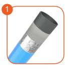
Solid construction made of black steel \$235JR, cleaned in the sandblasting process. Protected against corrosion by galvanizing and powder coating with polyester paint QUALICOAT attested.
