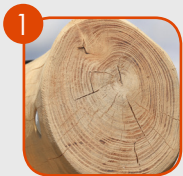
1 Posts are made of black locust.
