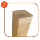
Soft conifer wood 90 x 90 mm, coreless, glued in layers with polyurethane glues, totally resistant to water. Wood posts processed in three-phased impregnation process.
