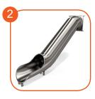
Tube slide made of stainless steel AISI 304. The metal sheet is 2 mm thick and the end section is finished with a band made of pipe 33,7 mm. The surface is polished.
