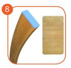
Bended posts made of soft conifer wood 9 cm thick, 26 cm wide and 280 cm long. The wood is glued in layers with polyurethane glues, totally resistant to water. Wood posts processed in three-phased impregnation process.
