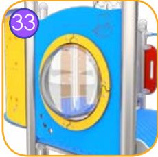
33 Hemispheric window with a diameter of 400 mm. Material: heat - formed polycarbonate 5 mm thick, resistant to vandalism.
