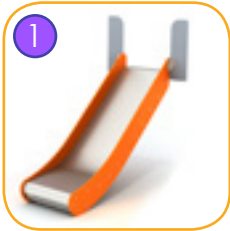
1 Slides made of stainless steel AISI 304. Metal sheet with a thickness of 2 mm formed in a CNC technique. Side panels made of HDPE polyethylene 15 mm, in the highest quality and totally damp-proof and resistant to UV.
