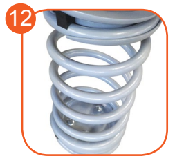
Springers' springs made of spring steel. The diameter of the spring is 200 mm and the diameter of the rod is 20 mm. The springs and the fastenings are galvanized and powder coated with polyester paint, UV resistant and QUALICOAT attested. The fastenings are designed especially for solutions used on a playground, so they are stripped of elements which can cause danger to children.
