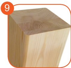
Soft conifer wood 140 x 140 mm, coreless, knotless, glued in layers with polyurethane glues, totally resistant to water. Wood posts processed in three-phased impregnation process.
