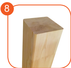
Soft conifer wood 90 x 90 mm, coreless, glued in layers with polyurethane glues, totally resistant to water. Wood posts processed in three-phased impregnation process.
