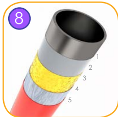
8 Solid construction made of black steel S235JR, cleaned in the sandblasting process. Protected against corrosion by galvanizing and powder coating with polyester paint QUALICOAT attested. 1 - steel, 2 - sandblasting, 3 - iron phosphatizing, 4 - zinc base, 5 - polyester powder paint.
