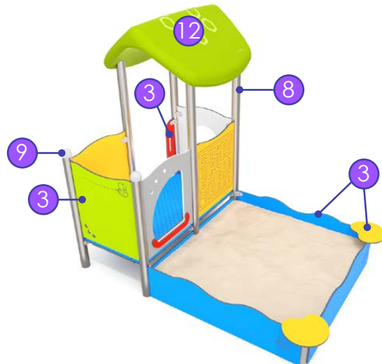
36 Passage module is made of 13 mm thick wood-like HPL, white and green 15mm HDPE boards and safe 8 mm thick polycarbonate.
