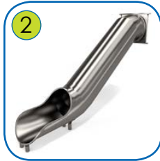
Tube slide made of stainless steel AISI 304. The metal sheet is 2 mm thick and the end section is finished with a band made of pipe 33.7 mm. The surface is polished.
