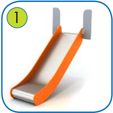
Slides made of stainless steel AISI 304. Metal sheet with a thickness of 2 mm formed in a CNC technique. Side panels made of HDPE polyethylene 15 mm, in the highest quality and totally damp-proof and resistant to UV.
