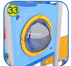
33 Hemispheric window with a diameter of 400 mm. Material: heat - formed polycarbonate 5 mm thick, resistant to vandalism.
