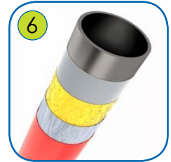
Solid construction made of black steel S235JR, cleaned in the sandblasting process. Protected against corrosion by galvanizing and powder coating with polyester paint QUALICOAT attested.
