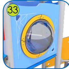
33 Hemispheric window with a diameter of 400 mm. Material: heat - formed polycarbonate 5 mm thick, resistant to vandalism.
